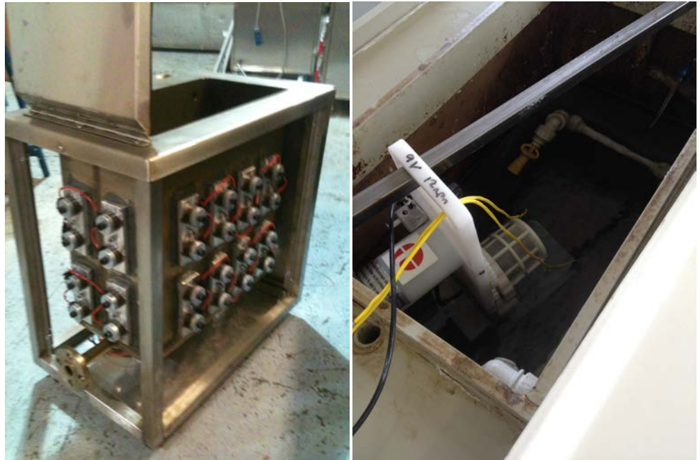
Ultrasound reactor showing the transducers (left) and barrel plating (right)
