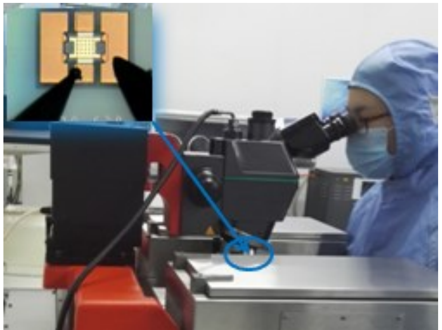
Fig.7 KGD testing during MEMS assembly for a satellite light phased array antenna (Courtesy of CAST).
