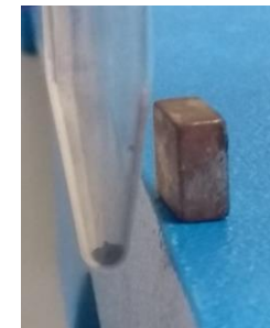
Test of magnetic properties of particles
