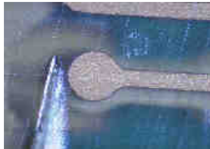
The images shows tracks leading to the blind via 0.020" capture pads and close up of pad just below the copper foil
