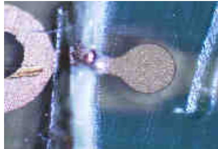
The images shows tracks leading to the blind via 0.020" capture pads and close up of pad just below the copper foil
