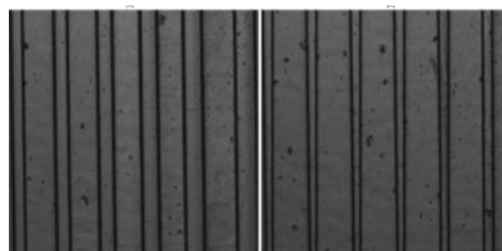
Fig.2: Photolithographically fabricated straight and tapered waveguides of a range of widths and taper ratios
