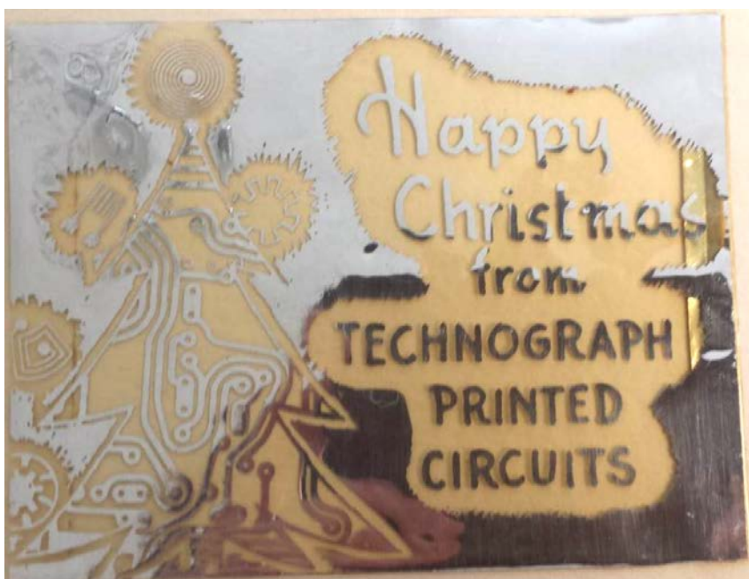
Christmas card of Technograph Printed Circuits made by the Printed Foil technique on clear paper
