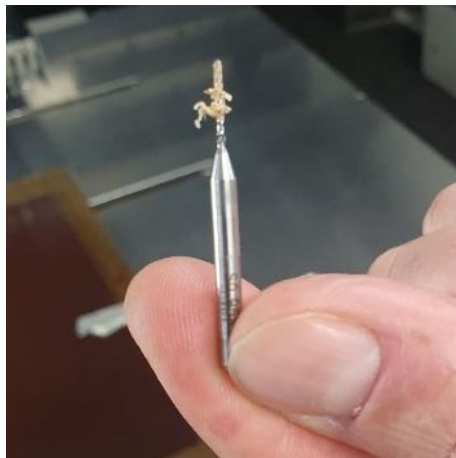
Acceptable drill bit condition
