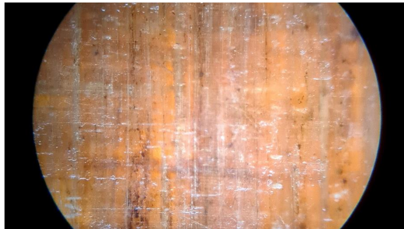
Improved fibre orientation + minimal bubbles
