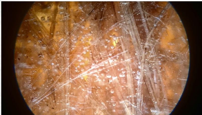
Stray fibres + polymer bubbles
